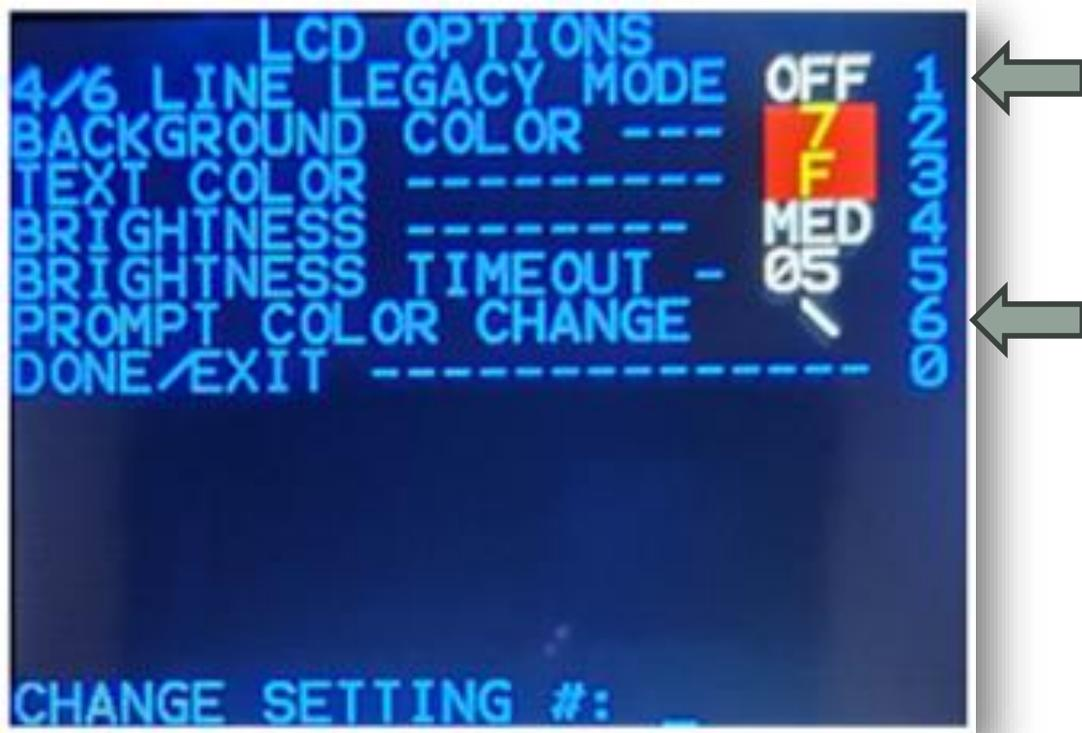
3. In the **LCD OPTIONS** screen, select option 1 to toggle **4/6 LINE LEGACY MODE** to **OFF**. This puts the unit into **15-line** mode.
